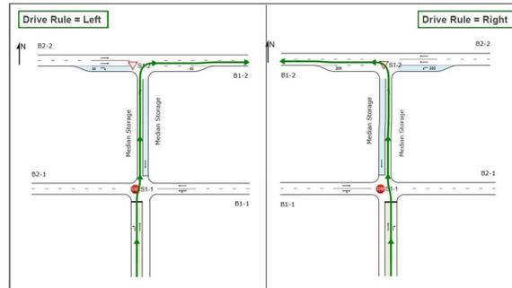
Figure 9.4.5.8 – Staged Crossing at T Intersection Type C-1 Network Template
